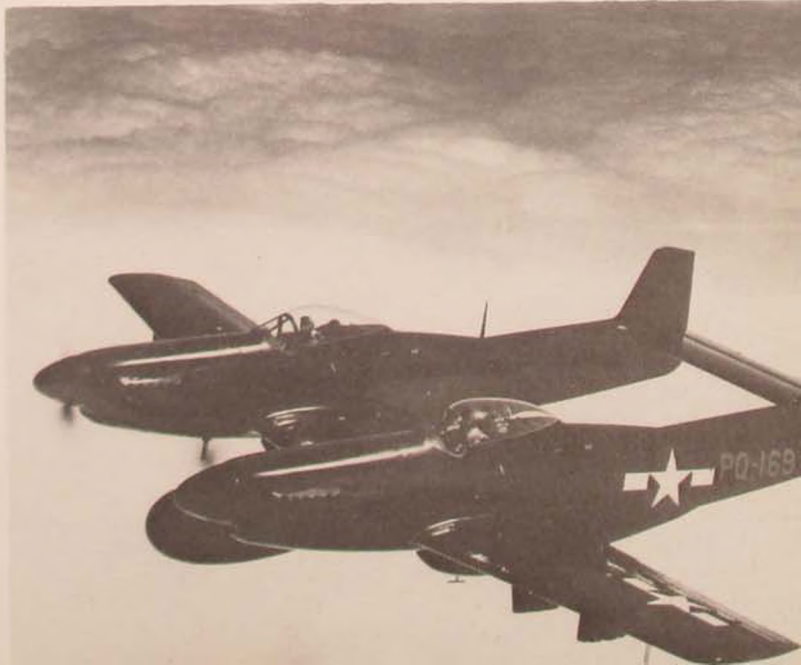
With the added weight and drag of radar for night interception, two engines were a must, and the design solutions were ingenious and varied. The twin-boom Northrop P-61 Black Widow (below, left) had some late World War II success in the Pacific as a night fighter; the F-82 Twin Mustang (right) was too late for World War II but saw limited use in Korea.
