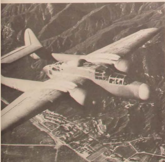
With the added weight and drag of radar for night interception, two engines were a must, and the design solutions were ingenious and varied. The twin-boom Northrop P-61 Black Widow (below, left) had some late World War II success in the Pacific as a night fighter; the F-82 Twin Mustang (right) was too late for World War II but saw limited use in Korea.
