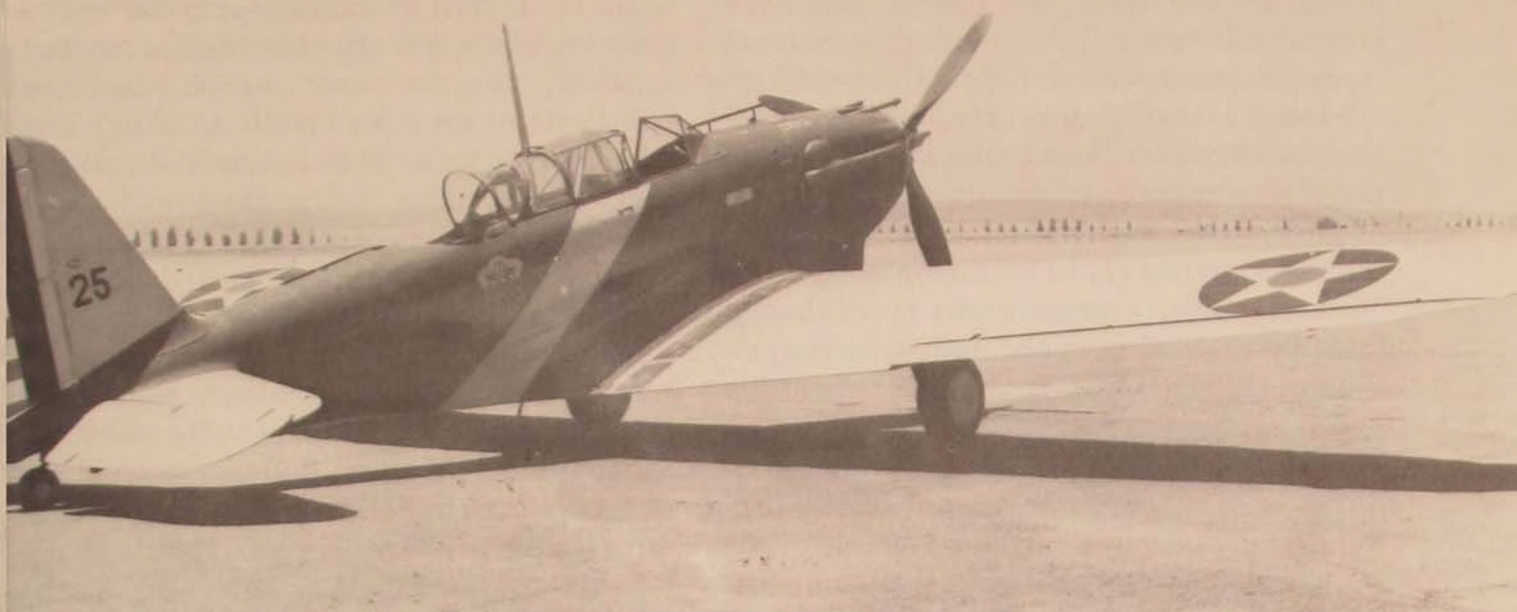
The last Air Corps fighter with a rearward-facing observer/gunner: the Consolidated PB-2A (above) at March Field, California, in 1937. . . . The need for streamlining reduced the gunner's field of fire, and a single .30 caliber machine gun (below) looked less and less of a threat at higher speeds and against all-metal airframes. The gunner could now communicate with his pilot by intercom.
